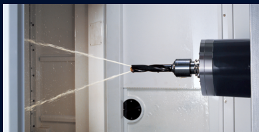
SPINDLE-THROUGH COOLANT (TSC) option
