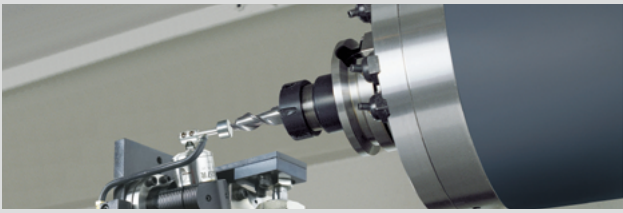
Automatic tool measuring device (TS 27R) option
